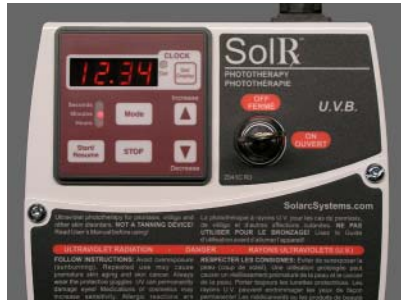
The digital timer and switchlock are important standard safety features.
