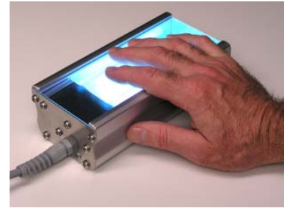
The lightweight aluminum body helps keep the device cool.
